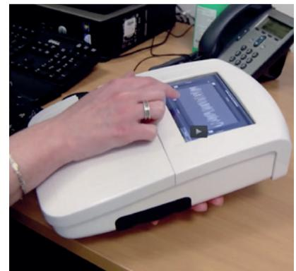
**The prototype “genetics lab in a box” which can sequence part of the genome and deliver results in just 15 minutes.**
